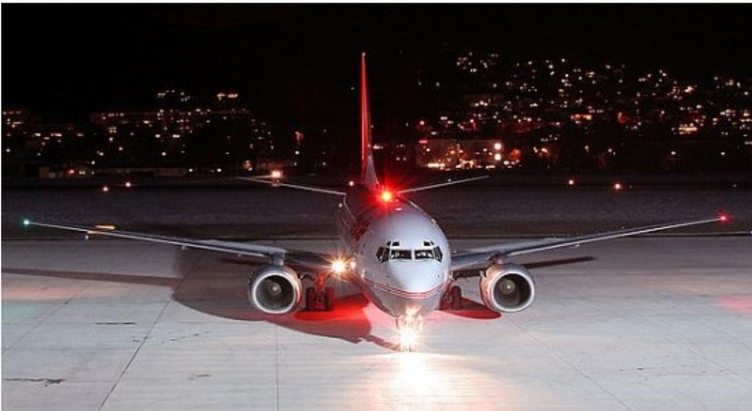
Notice the green and red lights on the wingtips. Notice the red flashing strobe light on the top of the jet fuselage (body). Notice the white lights on the front wheel and wing near the fuselage. If lights are on, there is power to the aircraft.
