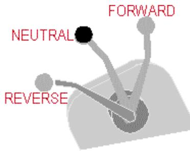
The clutches, with the black knobs, act like your gear shift. When the lever is standing straight up in the middle you are in neutral. When you push the lever forward you are engaging the forward gear and when you pull the lever back you are engaging the reverse gear.
