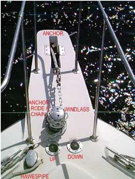
Normally, when underway the main breaker to the windlass will be turned on but there is usually a switch in the cockpit which disables the power temporarily. This is so that you don't accidentally step on the up and down switches on the deck while underway or while handling lines on the bow. Make sure that the cockpit switch is on.
