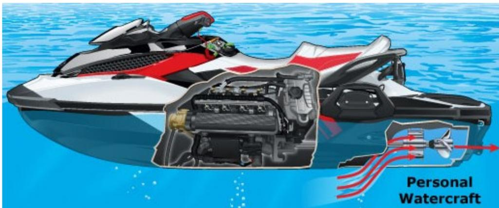
Notice the impeller is recessed inside the watercraft. A very strong jet of water exits out the back of the watercraft.
