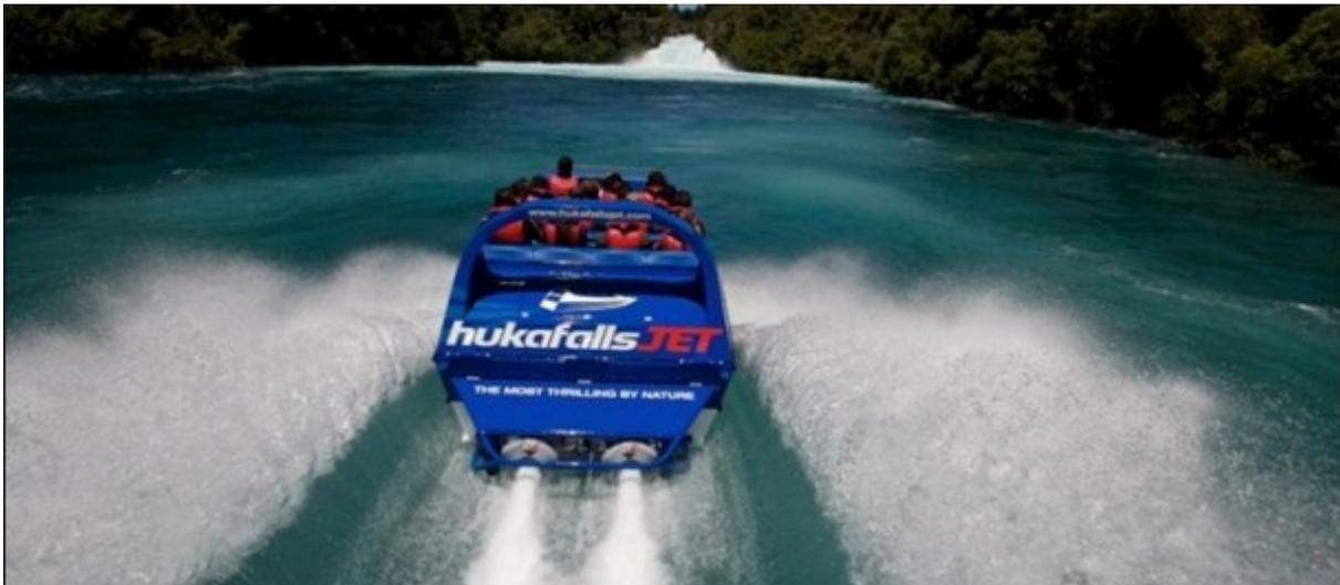
Notice the two high velocity water jets exiting out the back of this jet boat. It is very unpleasant to be hit by these jets. Stay away from this area.
