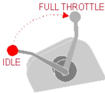
The throttles on a boat act like the accelerator on your car with one exception; *You shouldn't operate them with your feet.* The throttles, usually marked with RED knobs, are at idle when they are pulled all the way back toward you. As you move them forward, the fuel supply to the engine(s) is increased and, assuming you are in gear, you move faster.
