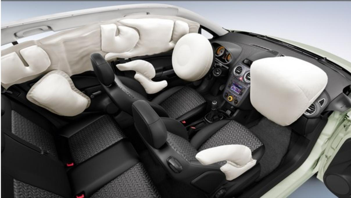
However, it should be understood that once a vehicle has suffered an impact, an airbag which did not go off or deploy DURING the accident, easily could go off AFTER the accident... when folks are not expecting it to. Always be aware and cautious of any airbag system that did not deploy if a vehicle has been damaged, it could go off and deploy unexpectedly.
