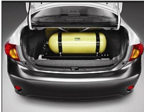
Honda with CNG (compressed natural gas) cylinder system
