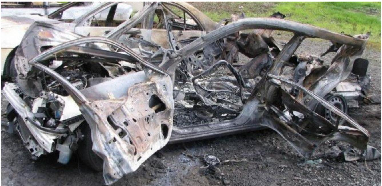
Honda after CNG cylinder explosion and fire.
