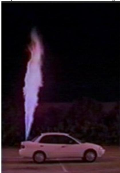
Hydrogen powered vehicle. Relief valve is venting and on fire.
