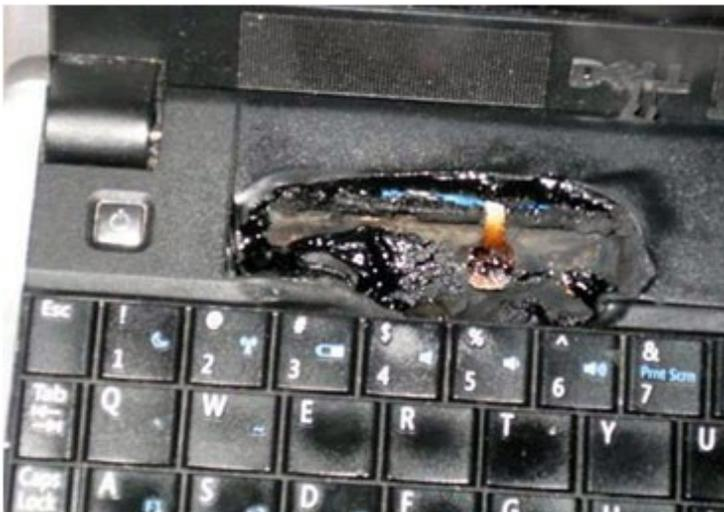
**Figure 1: Suspected Li-ion battery destroys laptop**
